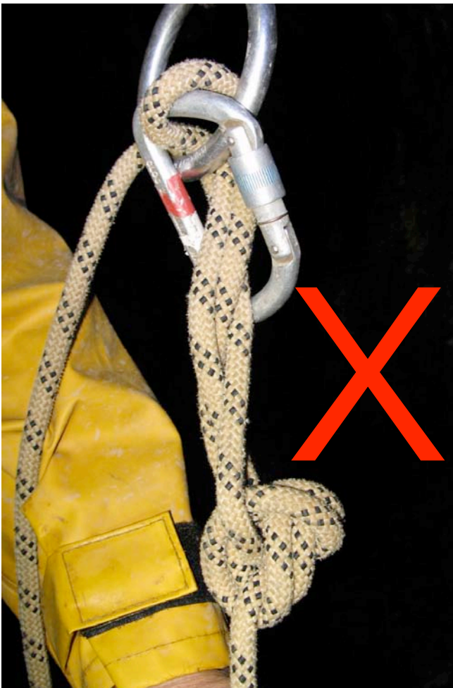
7. Long loop. Knot fed through karabiner. Now locks in both directions, i.e. no pull-back !!!
