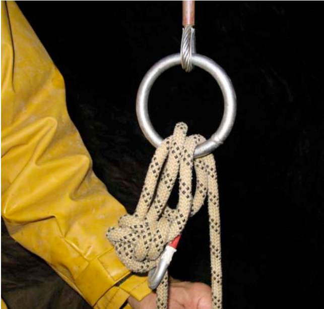
5. Fig.8 knot with long loop. Tension on live rope. Knot flipped through ring. Pull-back operates correctly.
